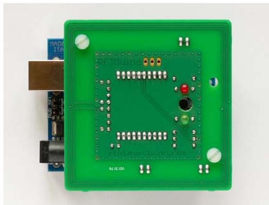
Fig 5. Mounted RFIDuino, top view
