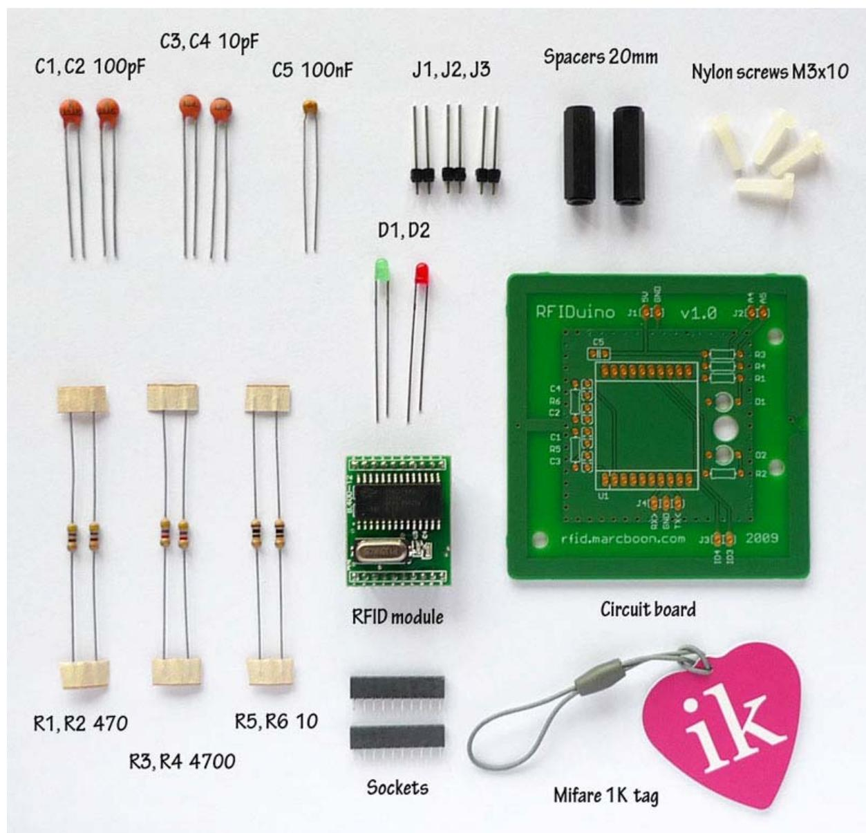
Fig. 2 - RFIDuino kit contents
