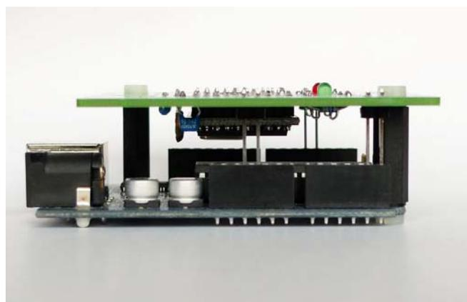
Fig 6. Mounted RFIDuino, side view
