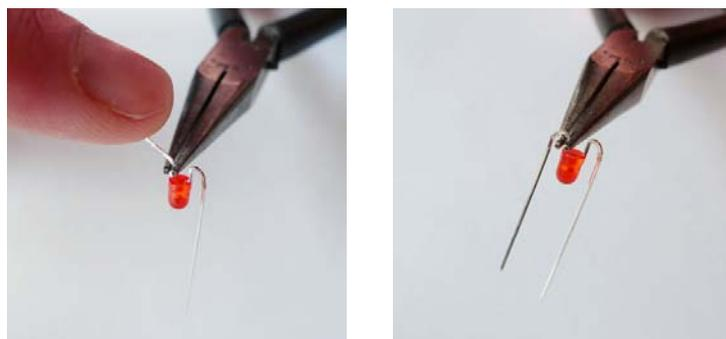
Fig. 3/4 - Bending the legs of the LEDs
